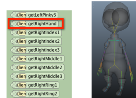
Figure A.8 Functions that link to an internal joint of an object
