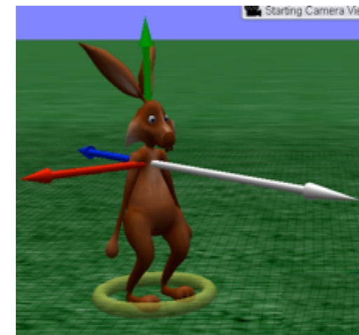
Figure 1 Orientation is defined by an object's sense of up and forward directions
