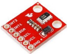
Figure 11-1. The MPL3115A2 on a Sparkfun breakout board
