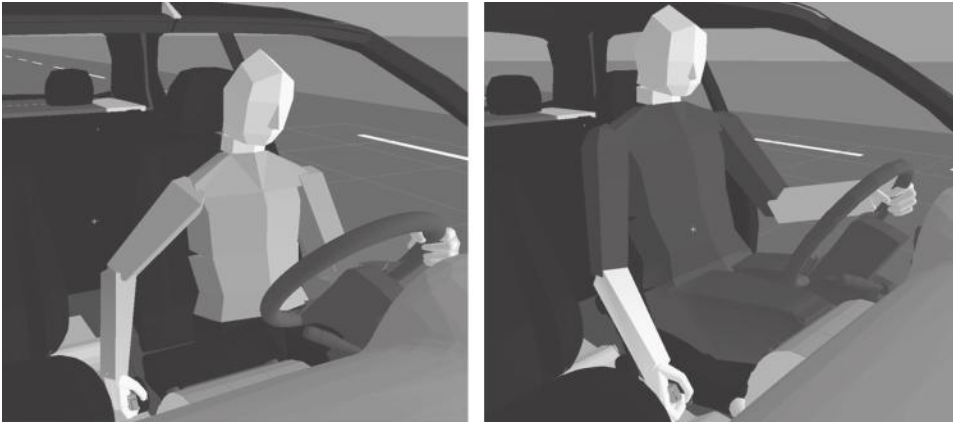
FIGURE 20.21 Reach to the handbrake for the smallest and largest accommodated drivers.
