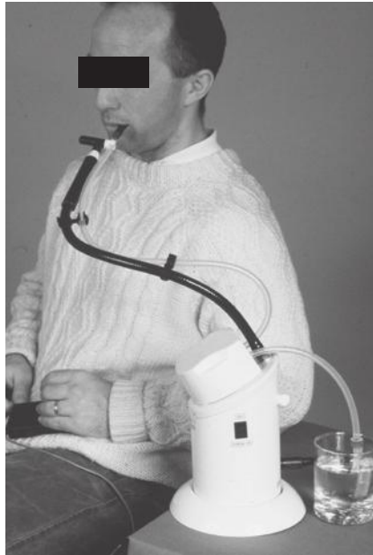
FIGURE 16.7 An automated drinking device, the Autosip, being tested by the author in 1992 at the Brunel Institute for Bioengineering.
