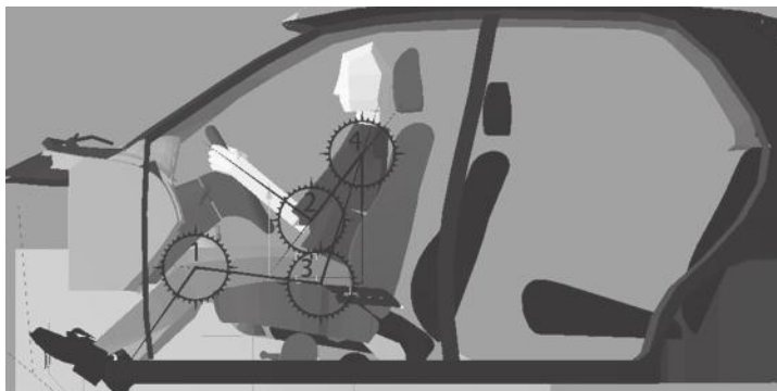
FIGURE 20.17 The minimum size of a driver that can be accommodated by the case study car.
