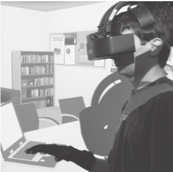
FIGURE 24.1 Image of a VR setting. Subject using HMD and a data glove, with image of VE behind him retroprojected.
