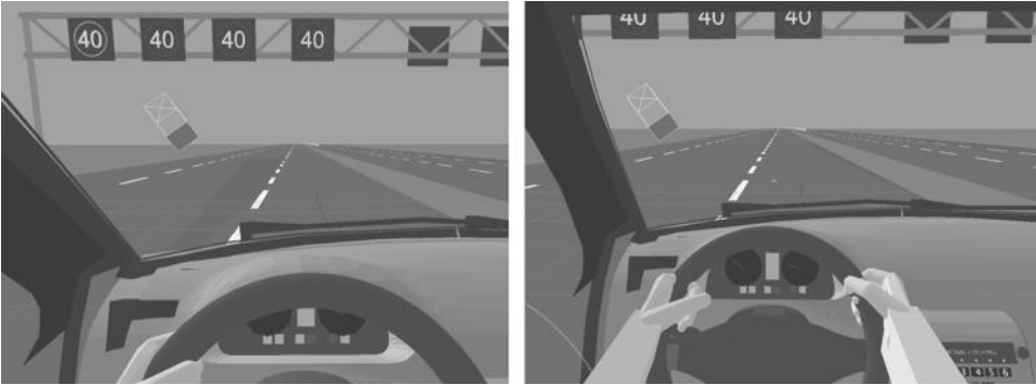
FIGURE 20.25 The visibility of the dials through the steering wheel in its highest adjustment setting.
