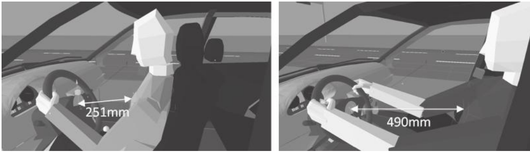
FIGURE 20.19 Clearances between the steering wheel and the chest of the human models.
