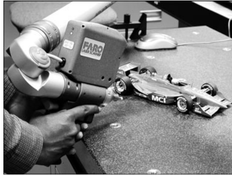
FIGURE 6.2.21 A car being laser scanned using a FARO Laser ScanArm. Images courtesy of FARO Technologies, Inc.
