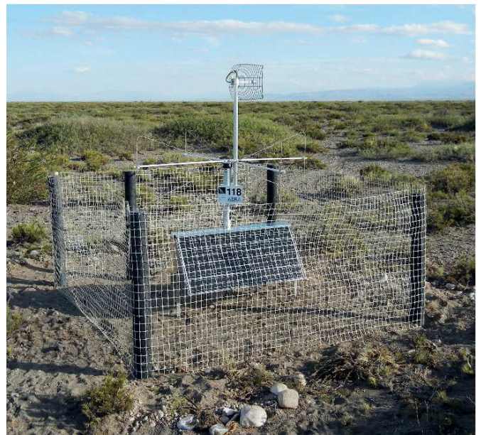
Figure 5: AERA station with Butterfly antenna.
