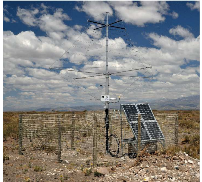
Figure 4: AERA station with logarithmic periodic dipole antenna (LPDA).
