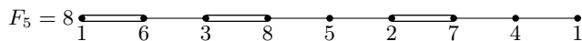
Figure 1: The periodically repeated block of the fifth approximant to the Fibonacci chain. Weak couplings t_w are represented by a single line, and strong couplings t_s by a double line. Below each site is its numbered label.
