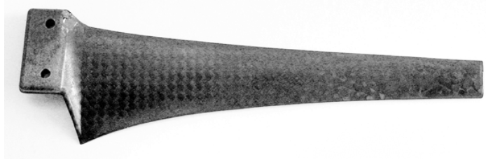
Figure 12: A near ideal rotor used on the ANU X4-Flyer. Rotor with optimum twist and chord with non-ideal geometry close to the hub [15, 16].
