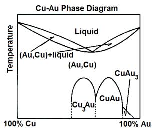
Fig. 1. Phase diagram Au/Cu
