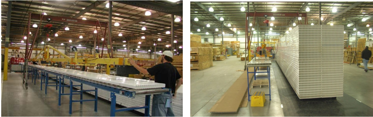
Figure 9: (a) The vacuum lifter, shown just above the extrusion, is supported by a movable gantry. An electronic weight scale is attached just below the hoist, above the yellow frame. (b) The vacuum lifter is used to stack extrusions for transport to the module assembly factory.
