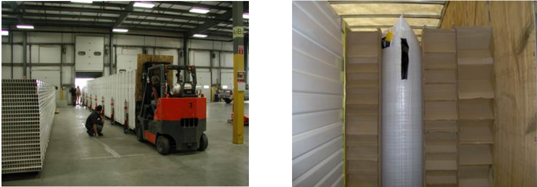
Figure 13: (a) A forklift was used to push one extrusion stack (2 x 28 extrusions) into a standard “53-foot” covered trailer. (b) The stack was braced for shipment with corrugated cardboard and inflatable airbags.
