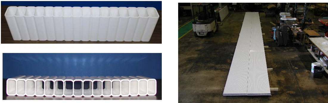
Figure 3: (a) Close-up photos of one 16-cell PVC extrusion, 15 cm long. (b) Two full-size 16-cell extrusions 15.5 m long placed side-by-side form the basis for an extrusion module.
