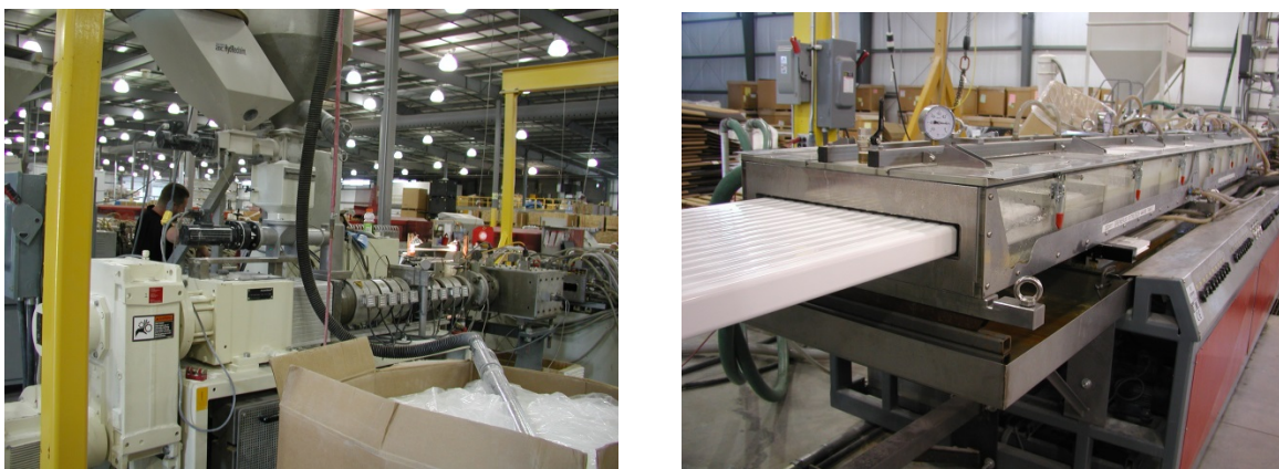
Figure 6: (a) N-27 powder is transported from a plastic-lined "gaylord" container into the extruder's hopper (top-center of the photo). The extruding barrel and back-side of the NOvA die (right-center of photo) are also visible. (b) Rigid extrusion exits the water cooling tanks and is about to enter the puller.
