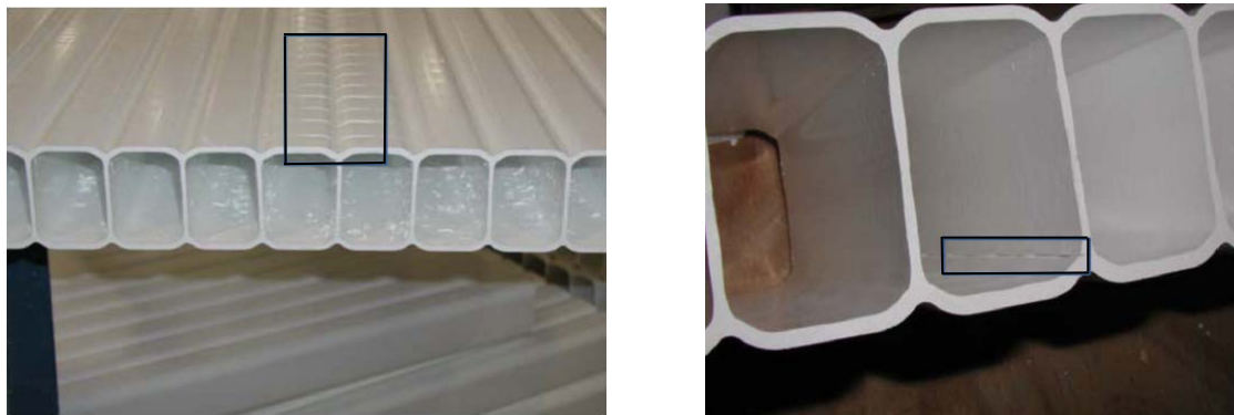
Figure 15: Example of extruding problems detected by visual inspection. Rectangular outlines added to the photos enclose (a) chatter marks on the top surface (b) a poor knit in lower right corner.
