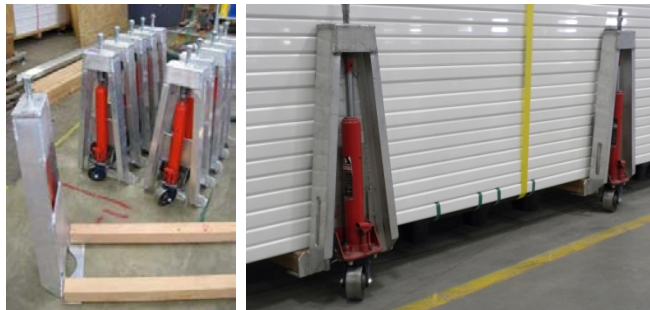
Figure 12: (a) Hydraulic caster jacks. (b) Jacks inserted under a stack of extrusions.
