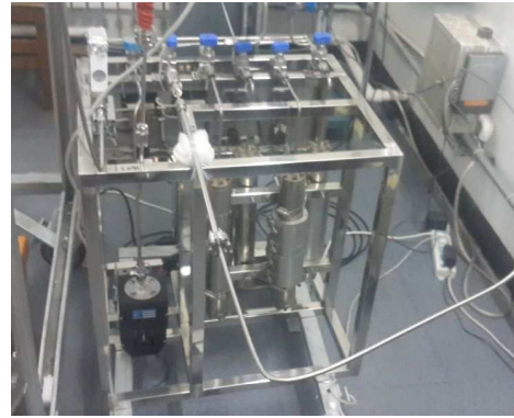
Fig. 3. The getter developed by Beijing Beiyang United Gas Co., Ltd is designed for reducing nitrogen, oxygen, and water impurities to lower than 0.1 ppm levels.
