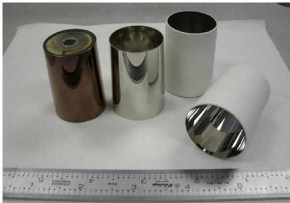
Figure 7. A test single-bounce conical mandrel, a NiCo shell, two NiCo ceramic hybrid shells from left to right. The width of the image spans about 14 cm.
