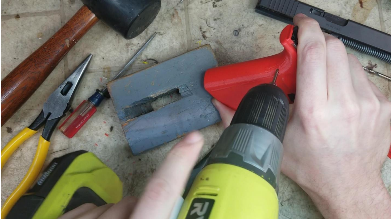
Recommended drilling technique. Hold the rail and block hard into the pocket. Drill gently and straight.
