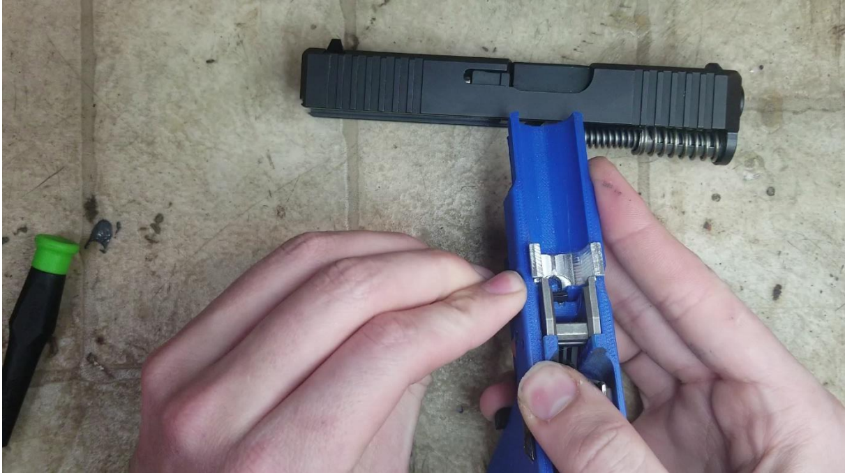
Pushing down spring with the latch
