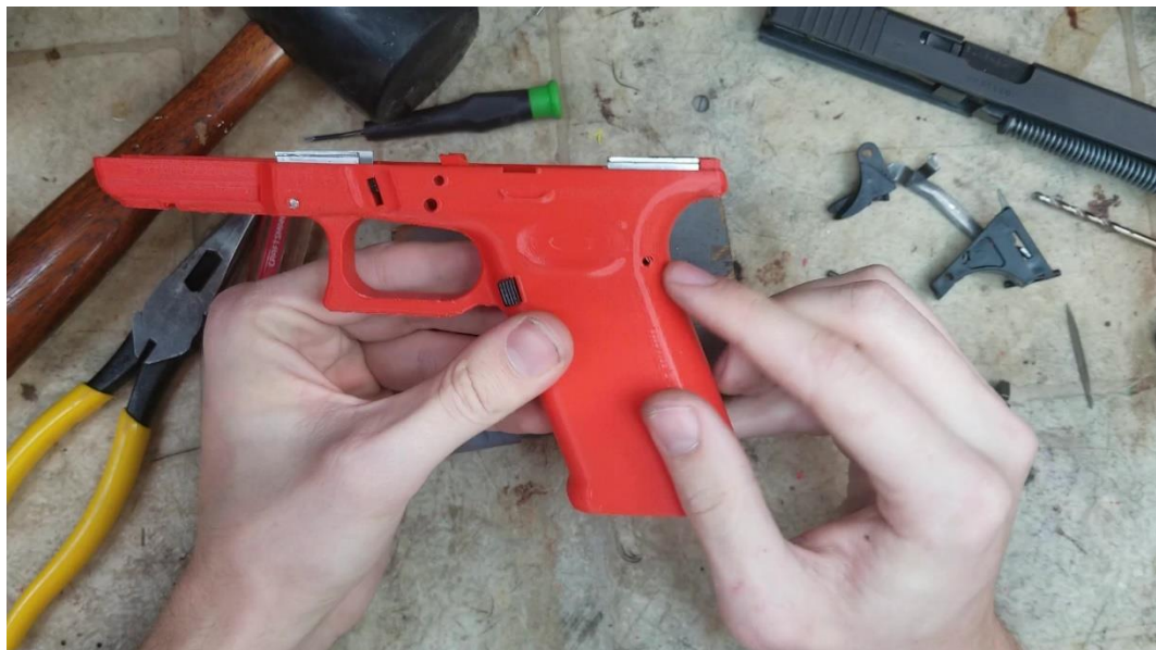
Rear rail installed. The pin hole should line up, or at least be very close to lining up.
