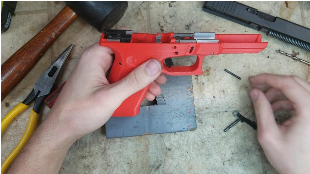
Locking block fully inserted.
