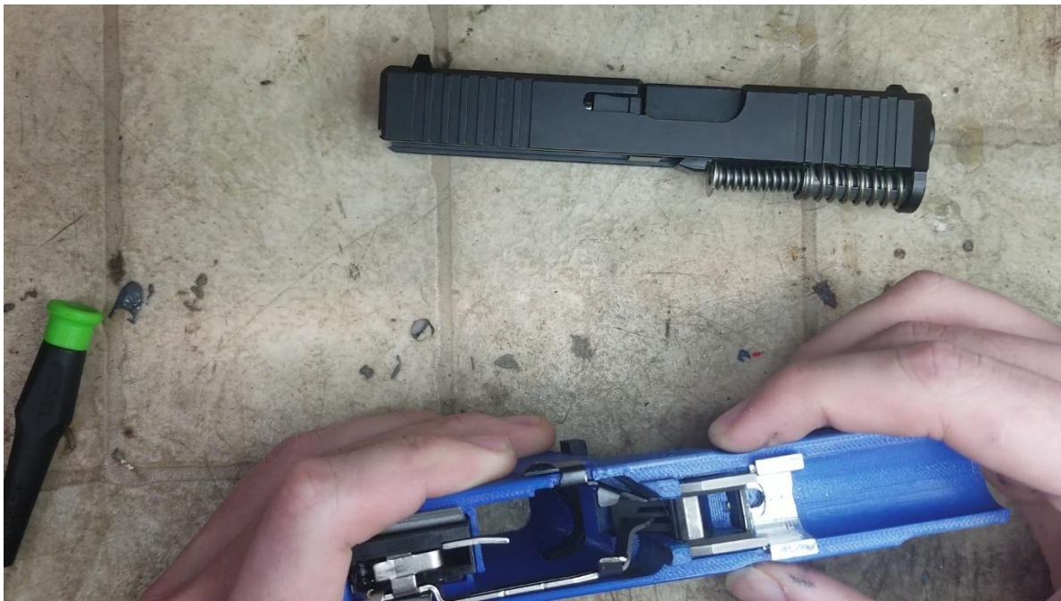
Slide latch pushed into the middle and held in by the spring. Wiggle the latch side to side to make sure the spring is holding it/you can't just push the latch out of the frame.
