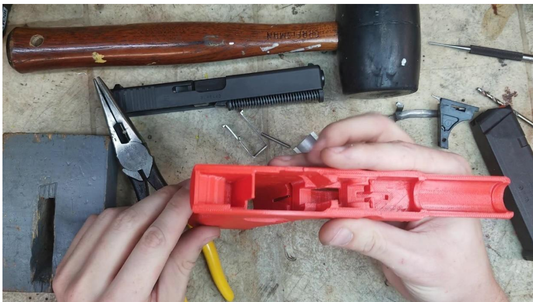
Mag catch spring fully inserted
