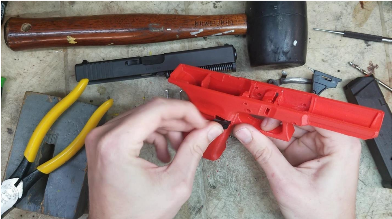
Test fitting the magazine catch
