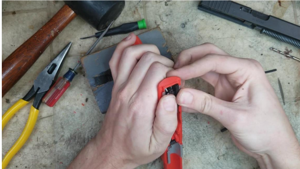
Push the rail and trigger block down firmly. The trigger bar and trigger should naturally fall into the frame.
