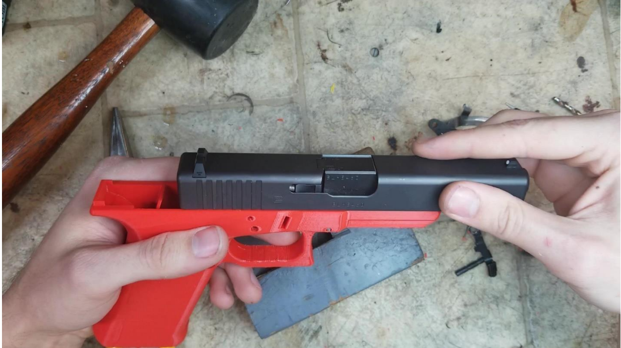
The slide should at least fit on this far without binding or dragging on the frame.
