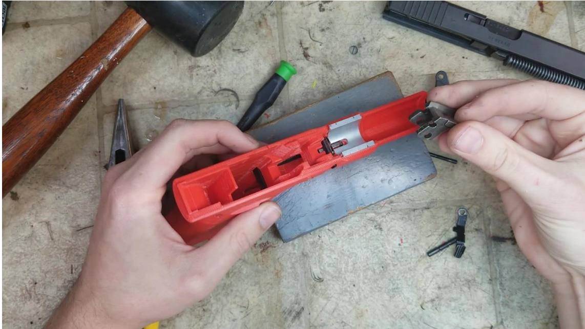
Locking block before installing
