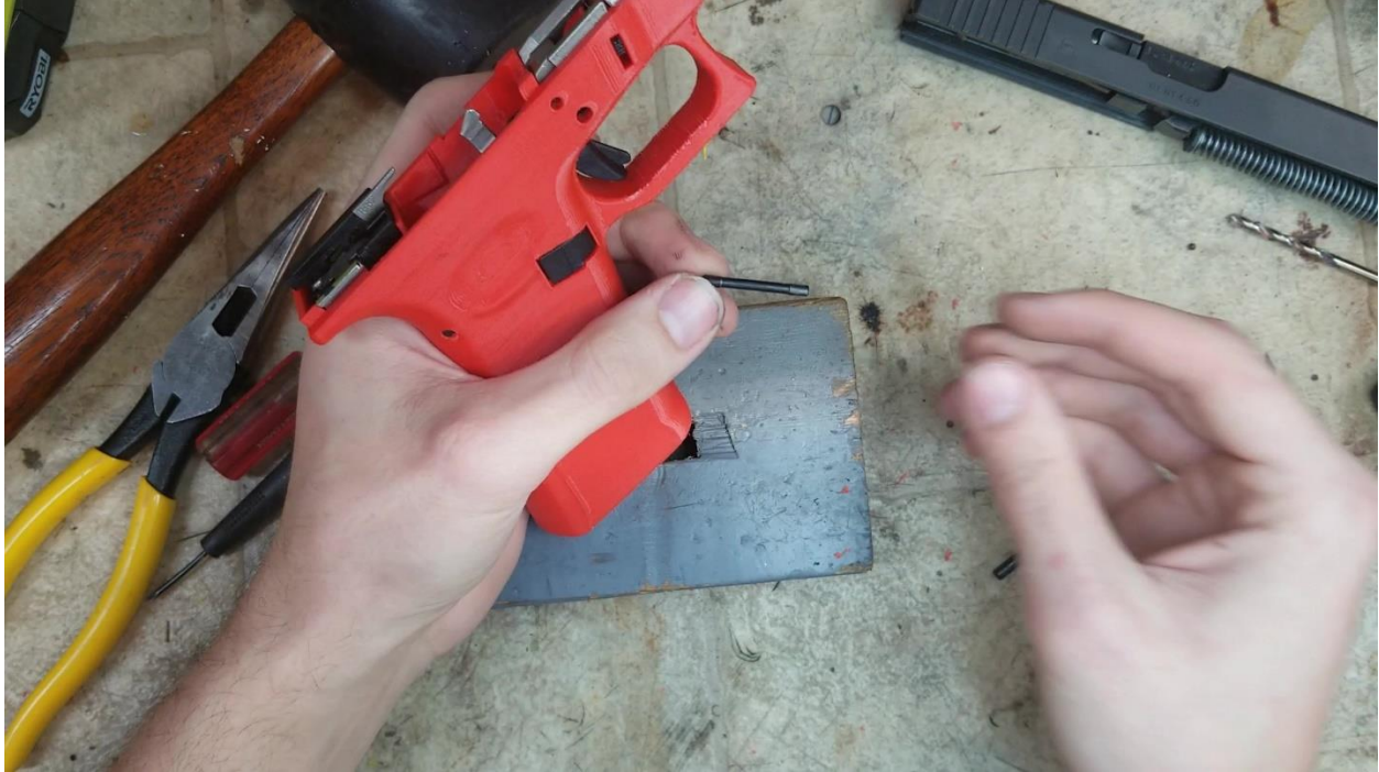
The correct pin to install in the TOP hole
