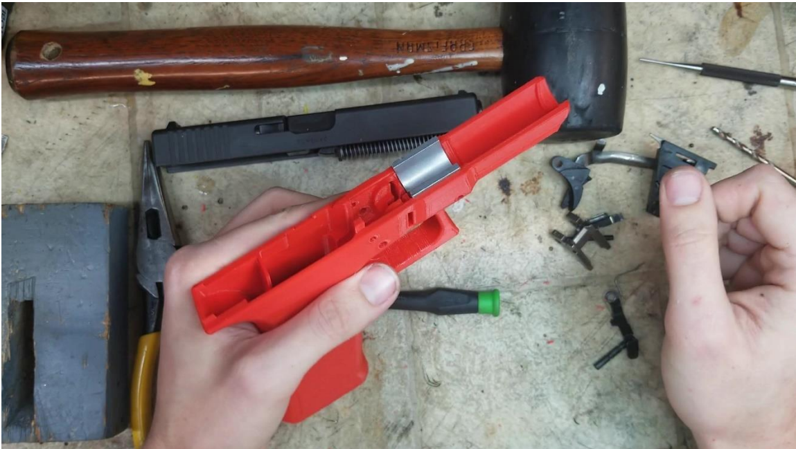
Front rail block placed in frame
