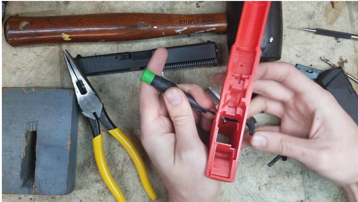
Moving spring past the mag catch while pushing the mag catch into the frame
