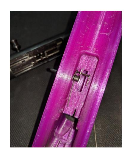
Drop in the trigger, and push the axes pin the rest of the way through. Make sure the disconnector Spring is under the pin. Then use a screwdriver to get the trigger Spring around the disconnector Axis pin.
