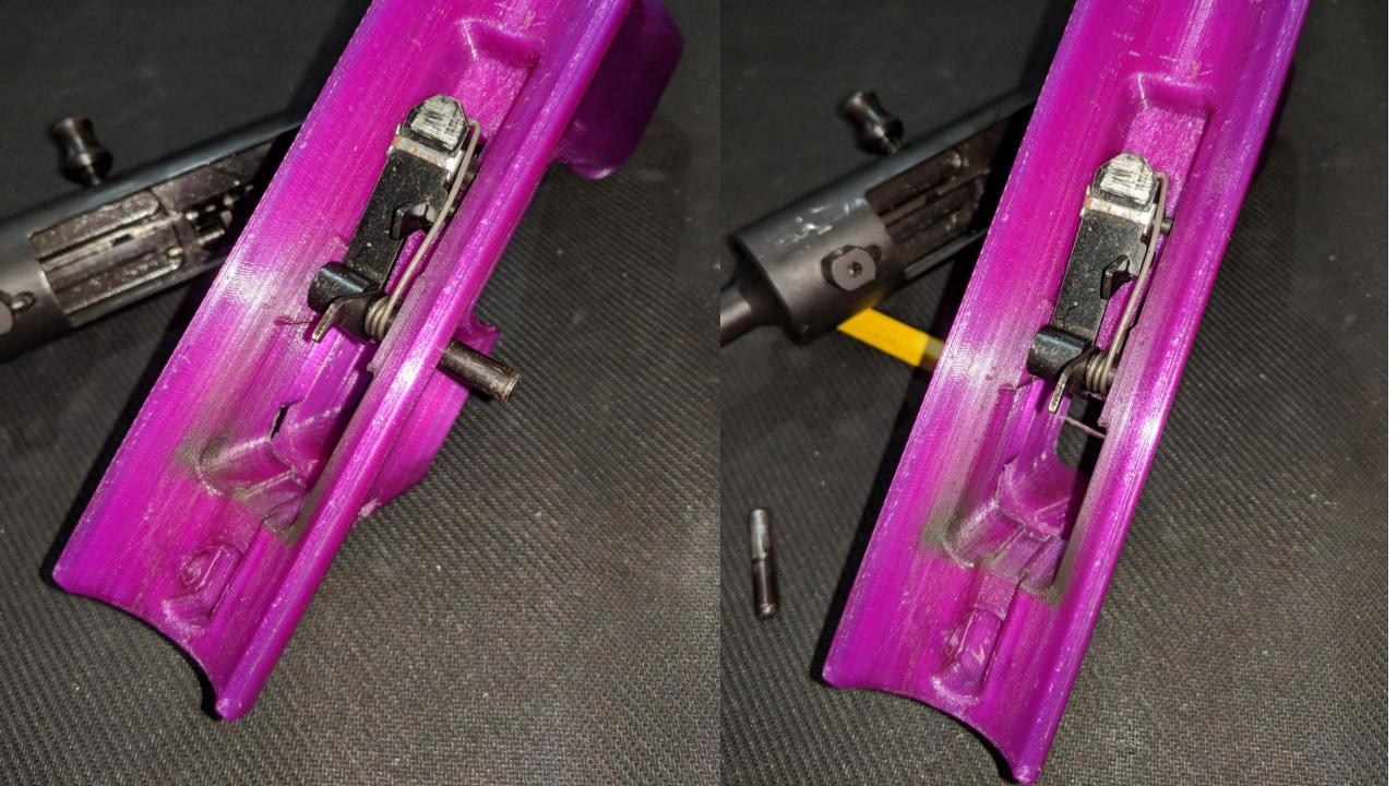
Line up the upper receiver and push the assembly pin through the lower and upper to secure them together. Applying oil to all pins before assembly will make less force required for tapping
