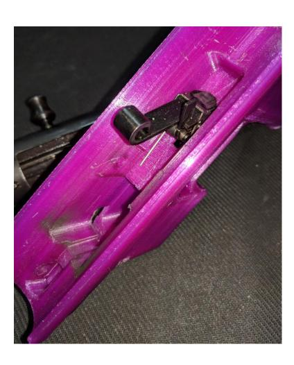
Hook the sear spring under the sear, then begin to push the sear axis pin through.
