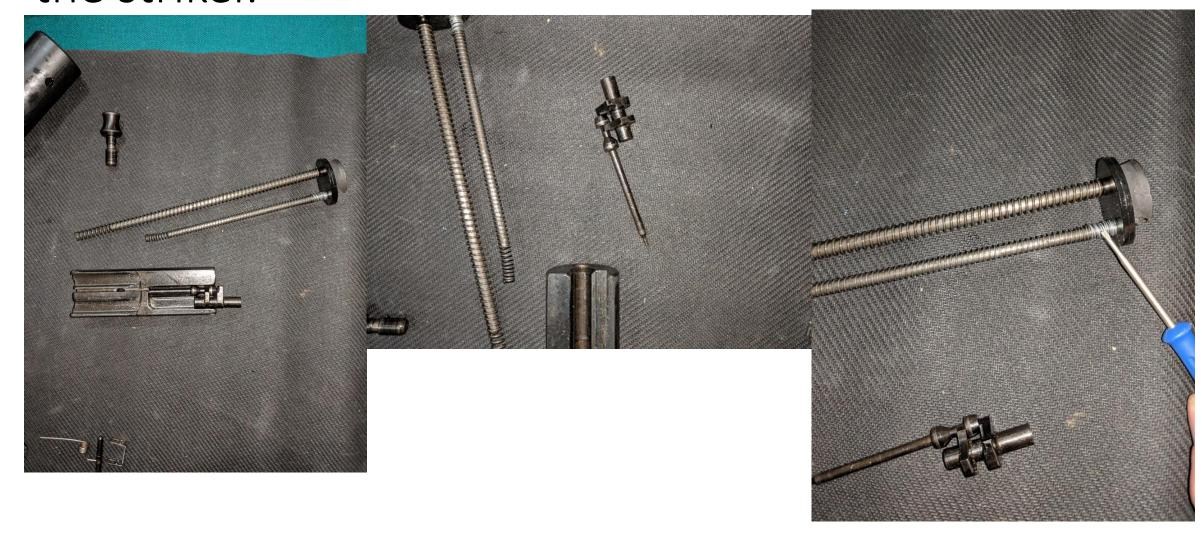
Insert the bolt into the upper receiver and lock it in by inserting the charging handle. After that simply screw on the end cap
