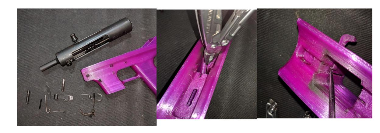
Insert the Trigger Axis pin, and slide on the Sear Retainer, and the Trigger Spring.
