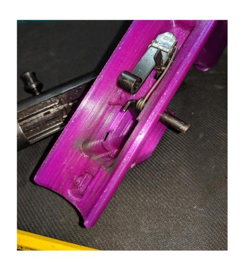
Put the pin through the lower hole that was drilled into the ejector before continuing to push the sear axis pin into the ejector.
