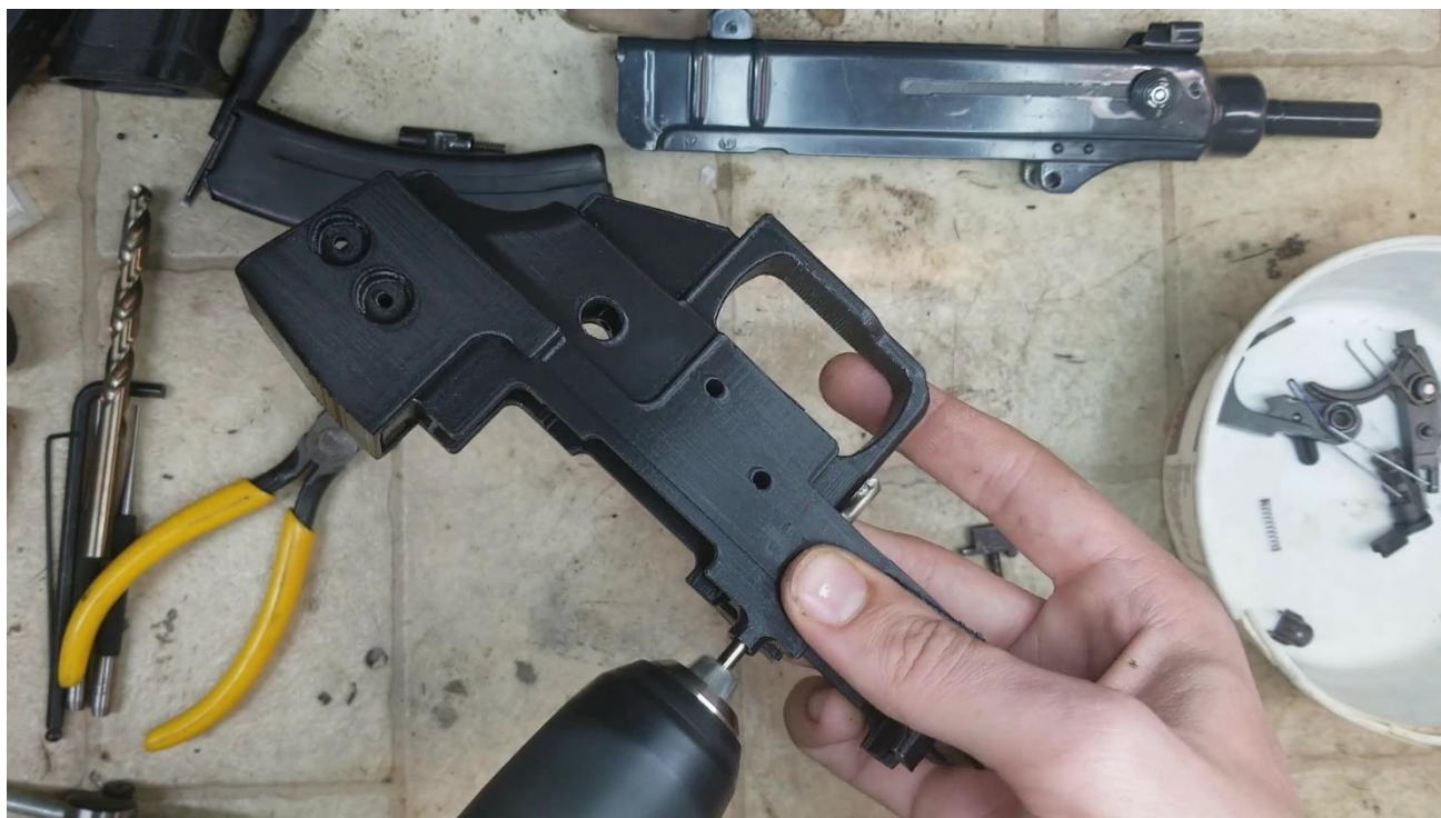
Bolt Catch Drilling
