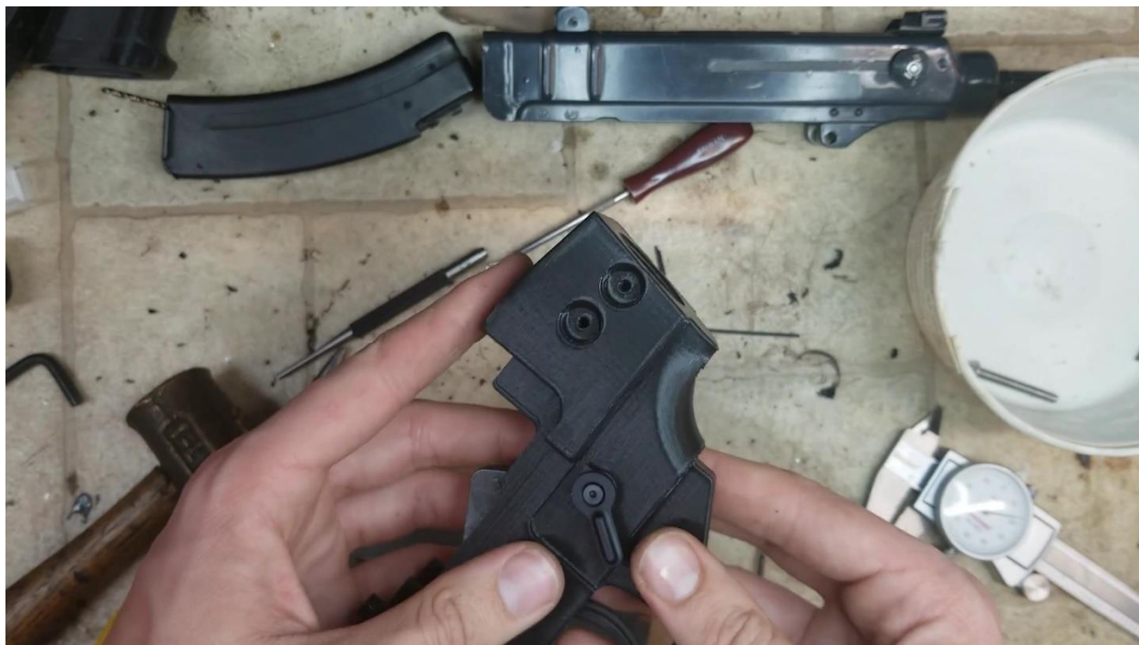
Installing Selector (Ensure it can Move Freely/Isn't Tight)
