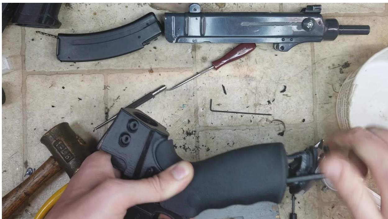
Installing Pistol Grip/Detent/Detent Spring
