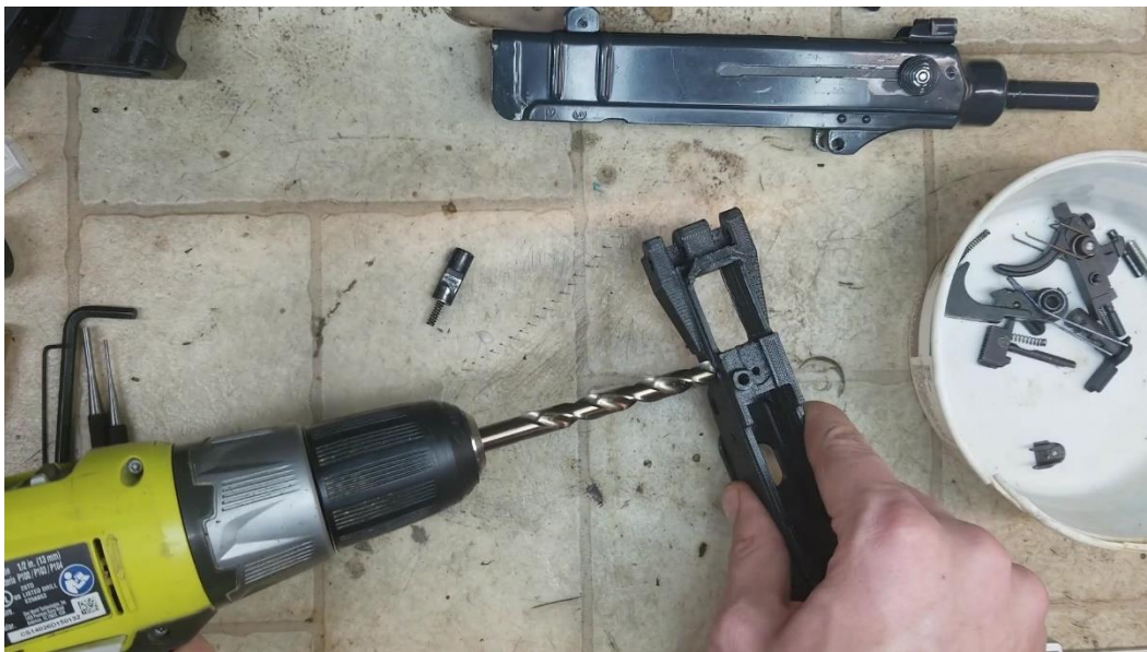
Magazine Catch Drilling
