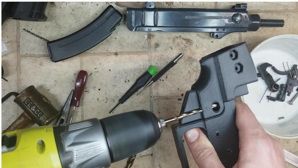
Drilling Selector Detent Hole
