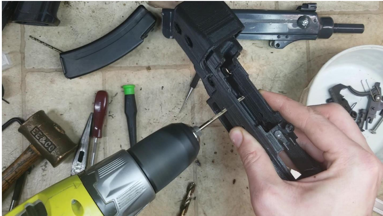
Drilling Fire Control Group Holes
