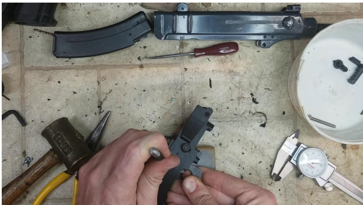
Installing Hammer and Trigger
