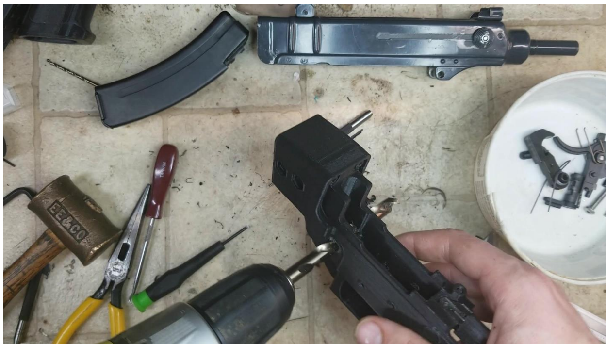
Drilling Selector Hole
