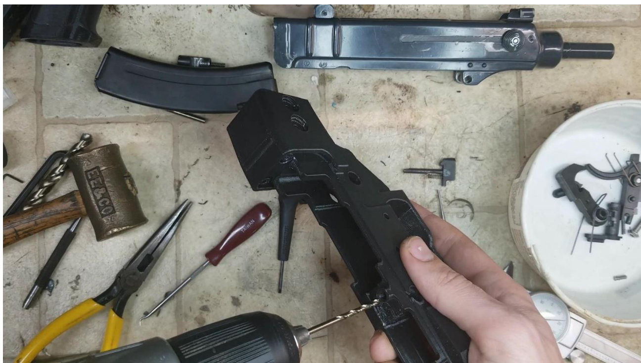
Plunger Drilling
