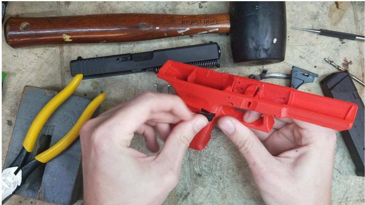
Test fitting the magazine catch
