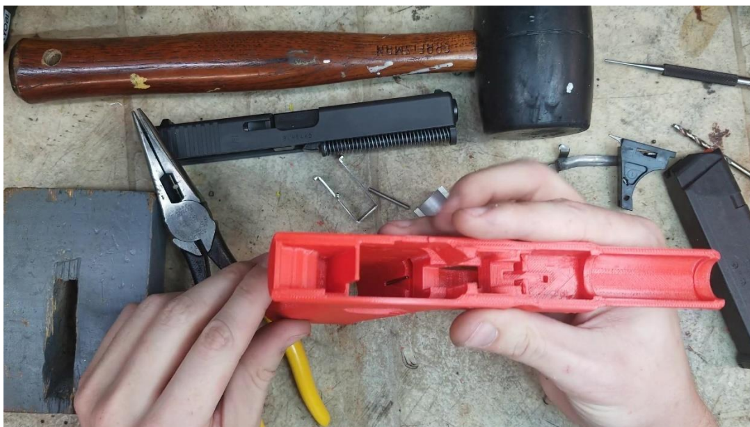
Mag catch spring fully inserted
