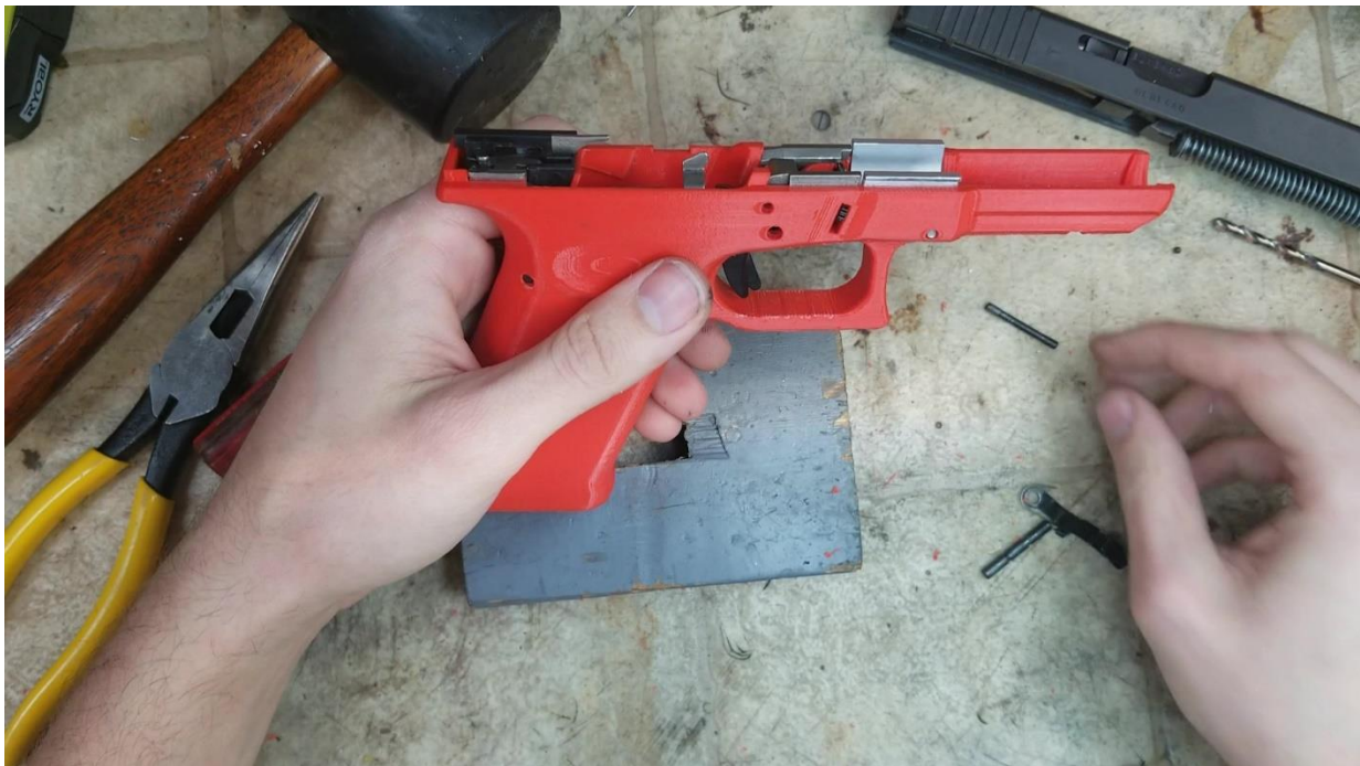
Locking block fully inserted.
